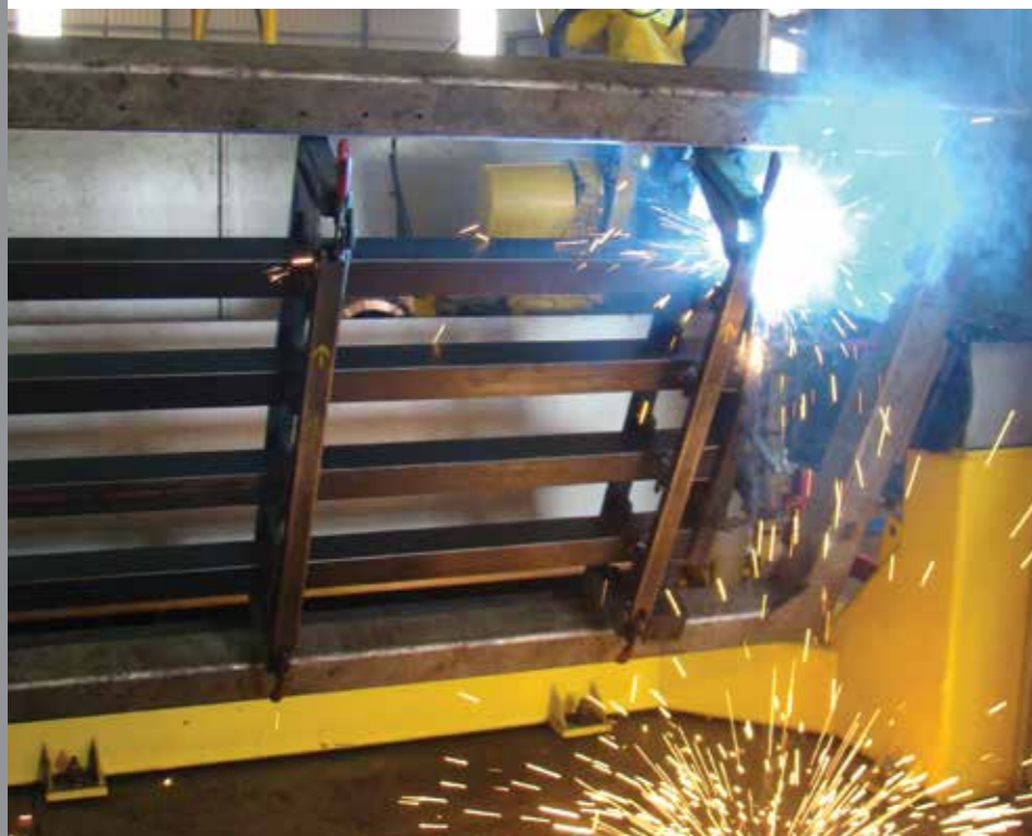
The support beams are made by deploying state-of-the-art technology such as robotised welding and quick-tightening tools, thereby ensuring the highest quality standards.
